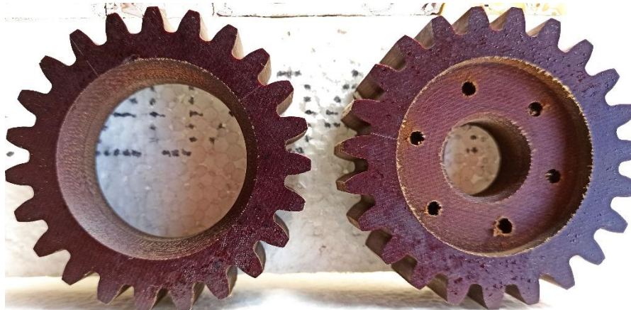
Fig. 3.10. Driven gear from the turret rotation mechanism of the BMP-1P
