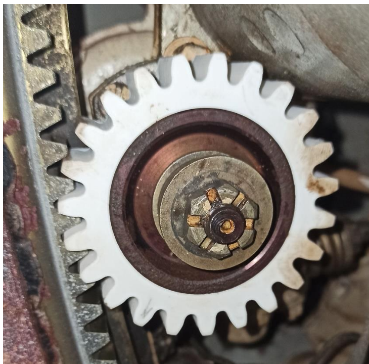
Фиг. 3.18. mounting a gear made of ABS
